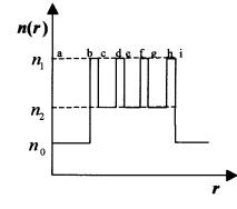
Fig. 1. Cross section of the hollow waveguide showing the hollow core and the dielectric films, also shown is the index of refraction profile in the radial direction.
