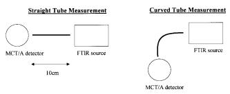
Fig. 3. Hollow tube transmission measurement setup on the spectrophotometer (FTIR).
