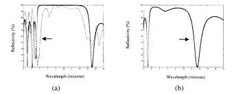
Fig. 2. (a) Measured (dashed) and calculated (dots) normal incidence reflectance for hollow waveguide in the radial direction. (b) Calculated grazing incidence reflectance for the TM mode.
