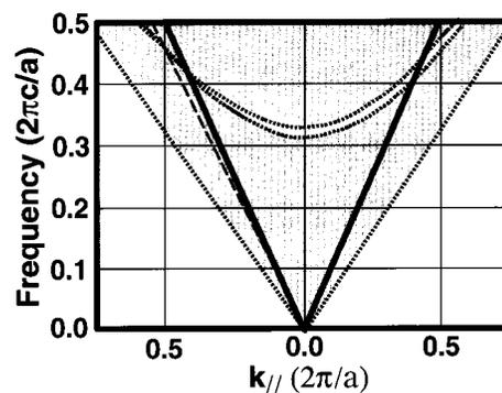
**Figure 3.** Photonic band structure of a multilayer film having the domain characteristics of the self-assembled polymer film. Shaded areas represent allowed propagation modes. Calculated using the transfer matrix method.<sup>17</sup> The Brewster line is represented by the narrow dashed line originating at  $k_{||} = 0$ . The light cone is outlined by the thicker lines representing the light line. Band edges are represented by dotted curves. Note: the Brewster's angle is  $46.5^\circ$ .
