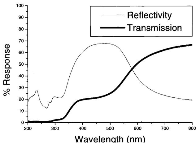
**Figure 1.** (a) Reflectivity spectrum of lamellar film showing a stop band over the 400–550 nm wavelength range. (b) Transmission spectrum of the same film showing the drop in transmission from the range of 350–550 nm due to the photonic band gap. The film exhibits approximately zero reflection and transmission below 330 nm due to the very strong UV absorption of the polymer.
