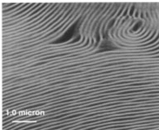
**Figure 2.** TEM micrograph of a microtomed cross section of the blend film. The isoprene is rendered white in this negative image due to  $\text{OsO}_4$  staining. Shown are regions of well-ordered lamellae as well as defects typical of the film.
