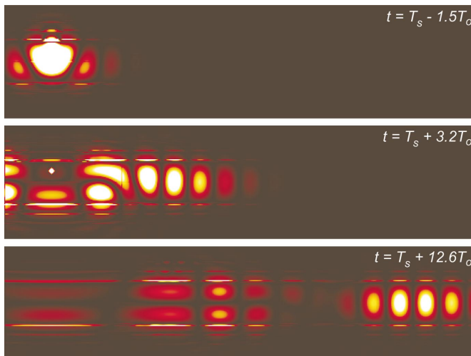
FIG. 14. (Color) Snapshots of the distribution of electrical power in the waveguide for a single-dipole source near the inner surface ( \rho = 1.2a , r_i = 2.144a ) pointing in the \theta direction.
